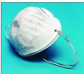
A respirator intended for use with general dust, doubled up to 'try' and give more protection is inadequate and should not be used.
