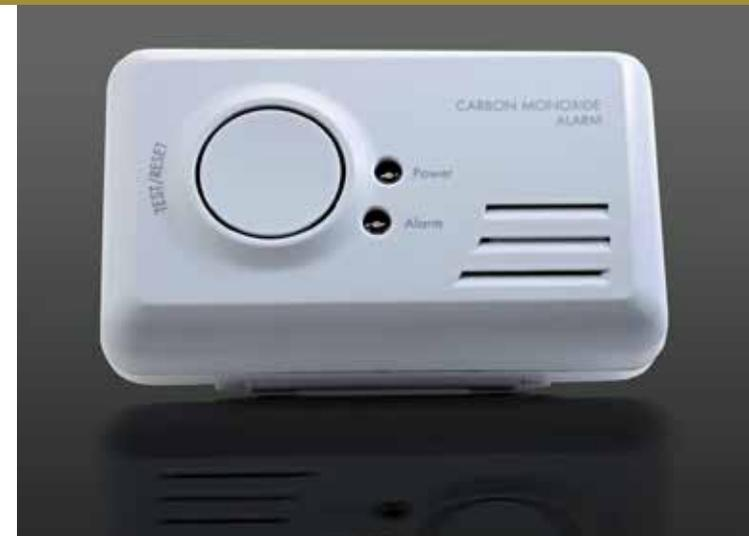
In all regions, a carbon monoxide detector (performing to British standard BS EN 50291) should be fitted in the same room as any new or replacement combustion appliance installation (such as a boiler), which is located in a building (including non-habitable areas) and not designed solely for cooking purposes\*.
