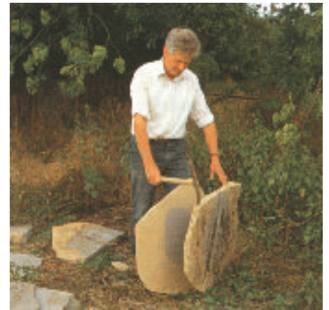
Figure 4 The rock is split along the bedding planes into a suitable thickness for roofing.
