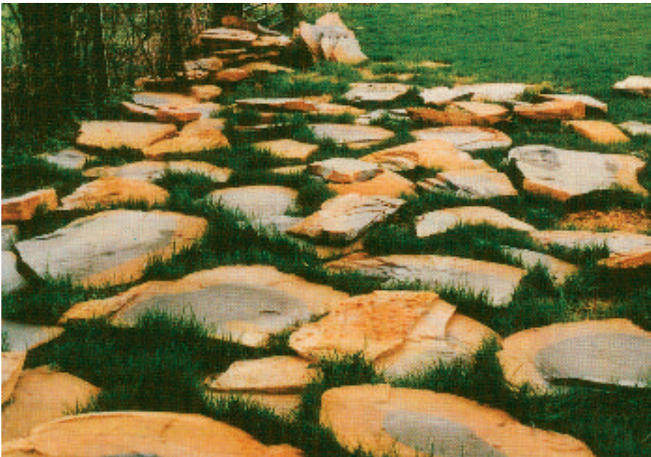
Figure 2 Collyweston, Northamptonshire: stone laid out for splitting by winter frost (Photograph: Daniel Martin)
