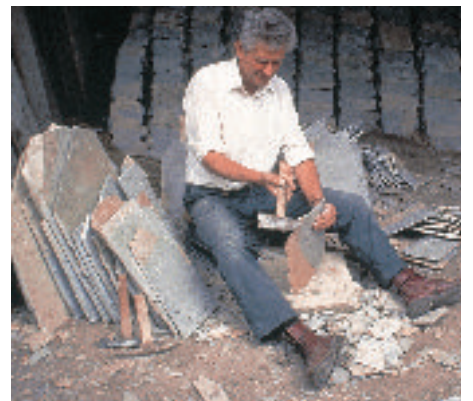
Figure 5 Once split to a suitable thickness, the stone is dressed roughly square and a fixing hole made.
