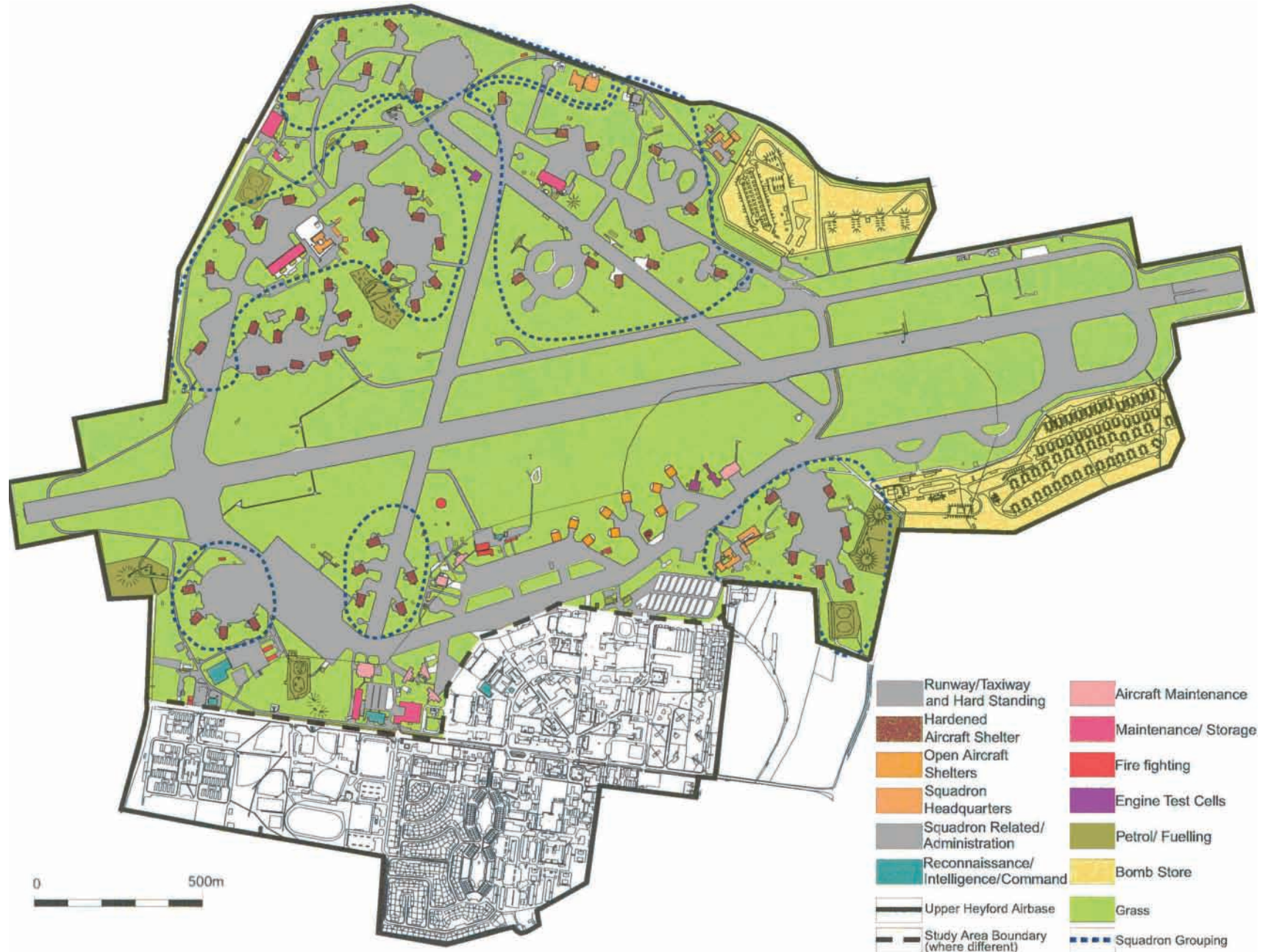
Figure 5: The functions of the buildings and structures on the flying field during the Cold War
