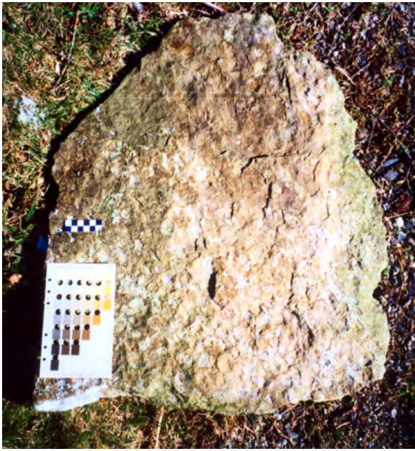
Fig. 11. Harnage stone-slates from near Acton Burnell in Shropshire were delved specifically to renew part of one roof. This established a source and method for conserving roofs, which represents too small a market to justify a permanent operation. Photo: Terry Hughes
