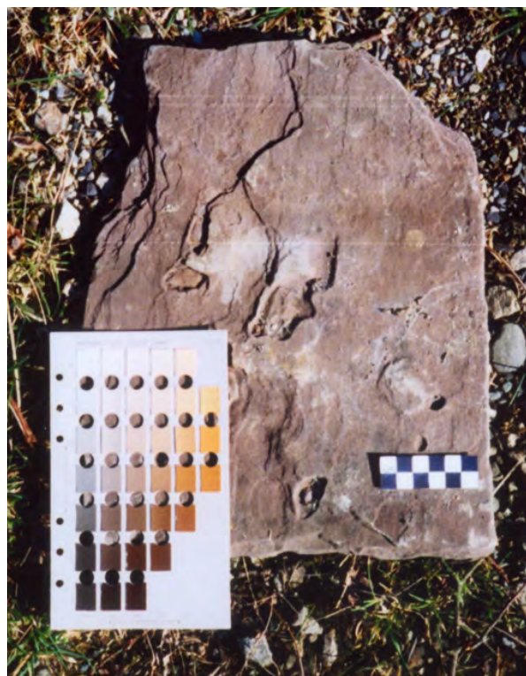
Fig. 16. A number of formations in the Old Red Sandstone in Herefordshire have been sources of stone-slates in a variety of colours from grey-green to red. Originally, roofs would have almost always been a single colour reflecting the nearest delph. Because of the decline of the industry many roofs are now a mix of differently coloured stone cannibalised from a variety of buildings. Photo: Terry Hughes
