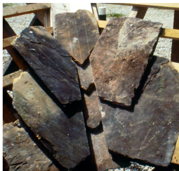
Fig. 48. Chevron valleys are traditional in the Pennine regions. A row of pointed stone-slates is laid up the valley and the adjacent slates on both sides are chosen or cut to mitre against the valley slate and to provide a half bond with the main slating. Photo: Terry Hughes.
